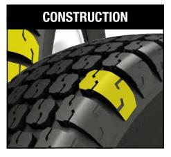
• The elongated lug at the shoulder wraps the tread around the sidewall and reduces the damage caused while turning on turf.
